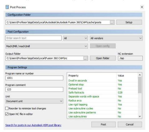
29. After all the settings, clicking on *Post* button opens a new window with the generated NC code, which we have to clean before we transfer it to the machine controller.
