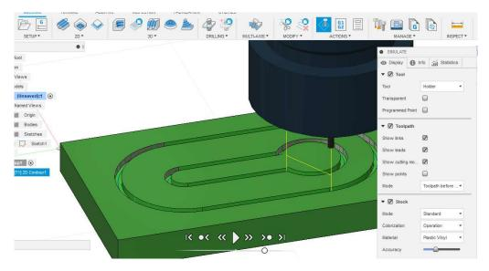
28. After reviewing the simulation, if no errors are shown, we can proceed to the generation of NC code through the *Post Process* option from the *Actions* menu. A window opens where we can choose the type of machine and the type of program on the computer.
