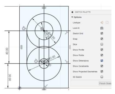
11. By using the *Trim* command it is possible to cut out part of lines or circles that we do not need anymore. If there are some auxiliary lines, we can select and delete them with the *Delete* key, which speeds up the deletion of lines or circles.
