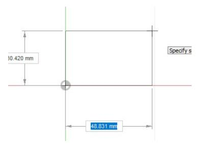
7. By using the *Sketch Dimension* command it is possible do define the length of line or a diameter of the circle and where we want to draw it, as well as make and show the exact dimensions from the coordinate system origin. If there are bisectors in the drawing, we can draw them as auxiliary lines for easier positioning of other lines or circles and delete them later.
