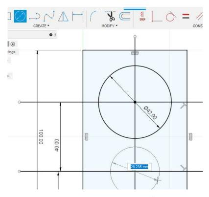
9. With the *Line* command it is possible to draw the contour of the model. We can draw all object lines at once. Using just a left mouse click, the command remains active, and we can draw the next desired line. With the *ESC* key we turn off the line command.
