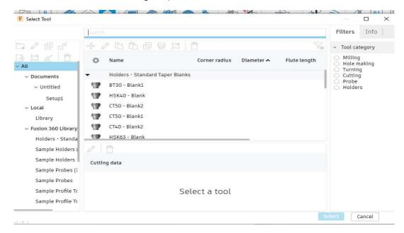
26. By clicking on the right mouse button over the option and selecting *Edit Tool* command we can change cutting tool and tool holder dimensions.
