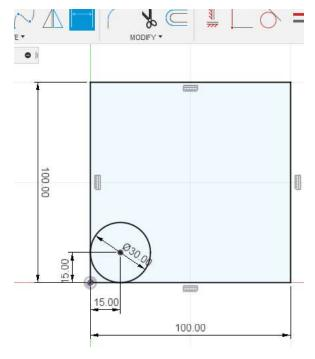
9. With the *Line* command it is possible to draw the contour of the model. We can draw all object lines at once. Using just a left mouse click, the command remains active, and we can draw the next desired line. With the *ESC* key we turn off the line command.
