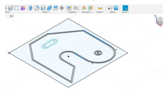
16. With the *Extrude* command we build the 3D model (pull the surface into space). It is necessary to choose closed surfaces. By entering the values or by pulling the blue arrow we define the thickness of the border.
