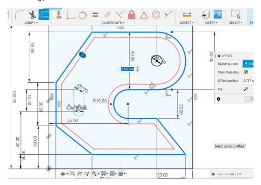
13. If all needed parts of a model are drawn, to create the 3D model it is necessary to exit from the sketch mode (*Finish Sketch* command). To apply *Extrude* or *Revolve* commands all the surfaces have to be closed (all lines connected).
