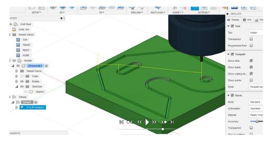
27. After reviewing the simulation, if no errors are shown, we can proceed to the generation of NC code through the *Post Process* option from the *Actions* menu. A window opens where we can choose the type of machine and the type of program on the computer.
