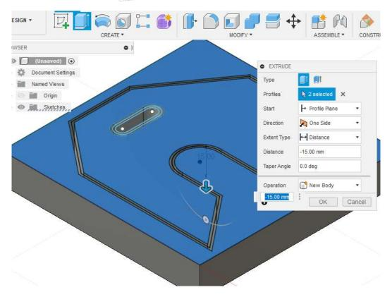
17. By using the *Point* command we define starting and ending point for simulation and generation of NC code.
