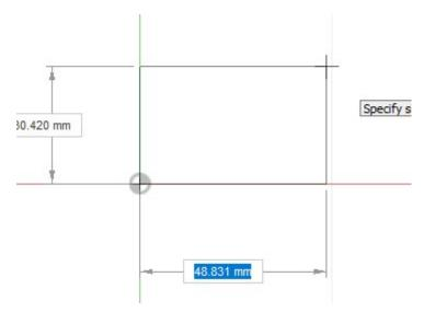
7. With the *Line* command it is possible to draw the contour of the model. We can draw all object lines at once. Using just a left mouse click, the command remains active, and we can draw the next desired line. With the *ESC* key we turn off the line command.
