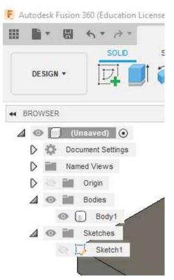
19. From the *Design* menu, by choosing the *Manufacture* option, it is possible to switch to the mode for making of the simulation and generating the NC code.
