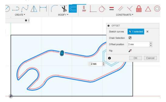
17. If all needed parts of a model are drawn, to create the 3D model it is necessary to exit from the sketch mode (*Finish Sketch* command). To apply *Extrude* or *Revolve* commands all the surfaces have to be closed (all lines connected).
