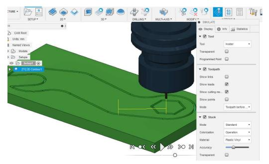
31. After reviewing the simulation, if no errors are shown, we can proceed to the generation of NC code through the *Post Process* option from the *Actions* menu. A window opens where we can choose the type of machine and the type of program on the computer.
