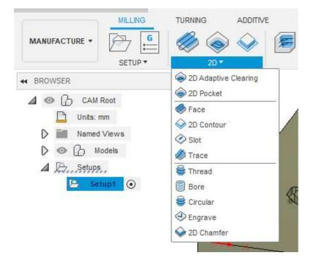
27. Choosing the *2D contour* milling option opens the window for setting up the cutting speed and ways of entering the cutting tool into the material. It is necessary to mark the contour on the 3D model. To finish the operation we need to choose the cutting tool.
