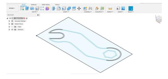
20. With the *Extrude* command we build the 3D model (pull the surface into space). It is necessary to choose closed surfaces. By entering the values or by pulling the blue arrow we define the thickness of the border.
