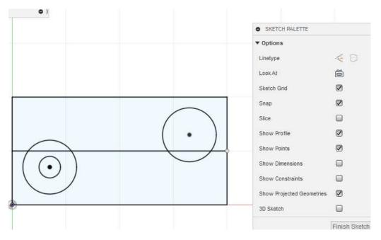
11. To draw a line tangent to a circle, we draw a line by moving the mouse when the tangent sign is present. Later, using the *Sketch Dimension* command, it is possible to determine the exact slope of the direction. Examples are shown in the following figures:
