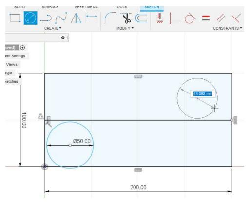
9. By using the *Sketch Dimension* command it is possible do define where we want to draw a circle as well as make and show the exact dimensions from the coordinate system origin.
