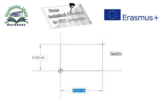
7. With the *Line* command it is possible to draw the contour of the model. We can draw all object lines at once. Using just a left mouse click, the command remains active, and we can draw the next desired line. With the *ESC* key we turn off the line command.
