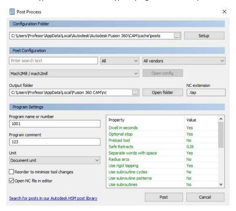
28. After all the settings, clicking on *Post* button opens a new window with the generated NC code, which we have to clean before we transfer it to the machine controller.
