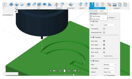
27. After reviewing the simulation, if no errors are shown, we can proceed to the generation of NC code through the *Post Process* option from the *Actions* menu. A window opens where we can choose the type of machine and the type of program on the computer.
