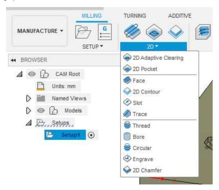
23. Choosing the **2D contour** milling option opens the window for setting up the cutting speed and ways of entering the cutting tool into the material. It is necessary to mark the contour on the 3D model. To finish the operation we need to choose the cutting tool.
