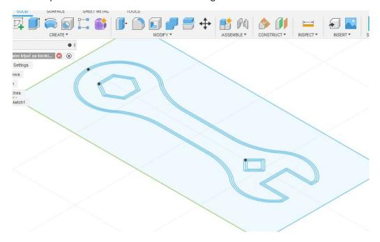
19. With the *Extrude* command we build the 3D model (pull the surface into space). It is necessary to choose closed surfaces. By entering the values or by pulling the blue arrow we define the thickness of the border.
