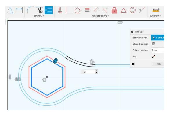
16. If all needed parts of a model are drawn, to create the 3D model it is necessary to exit from the sketch mode (*Finish Sketch* command). To apply *Extrude* or *Revolve* commands all the surfaces have to be closed (all lines connected).
