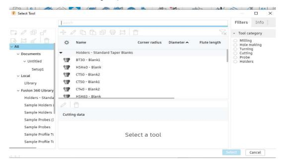
28. By clicking on the right mouse button over the option and selecting *Edit Tool* command we can change cutting tool and tool holder dimensions.
