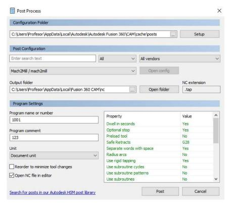
31. After all the settings, clicking on *Post* button opens a new window with the generated NC code, which we have to clean before we transfer it to the machine controller.
