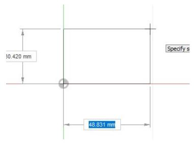
7. By using the *Sketch Dimension* command it is possible do define where we want to draw a circle as welll as make and show the exact dimensions from the coordinate system origin.
