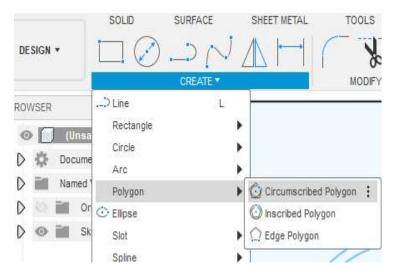
14. By entering the desired radius and number of vertices it is possible to draw the desired polygon.
