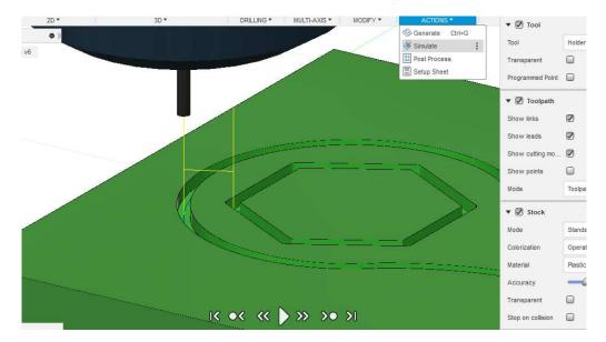
30. After reviewing the simulation, if no errors are shown, we can proceed to the generation of NC code through the *Post Process* option from the *Actions* menu. A window opens where we can choose the type of machine and the type of program on the computer.
