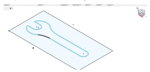
17. With the *Extrude* command we build the 3D model (pull the surface into space).
