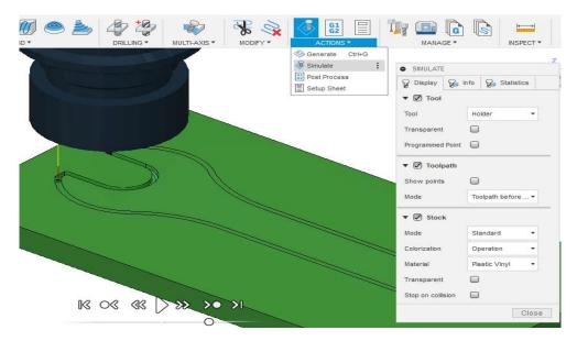
28. After reviewing the simulation, if no errors are shown, we can proceed to the generation of NC code through the *Post Process* option from the *Actions* menu. A window opens where we can choose the type of machine and the type of program on the computer.
