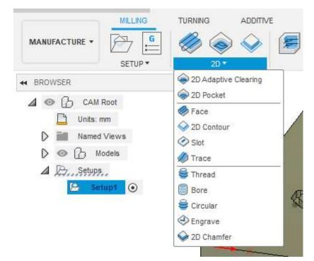
24. Choosing the *2D contour* milling option opens the window for setting up the cutting speed and ways of entering the cutting tool into the material. It is necessary to mark the contour on the 3D model. To finish the operation we need to choose the cutting tool.
