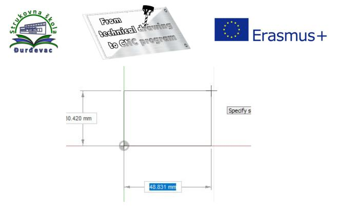
7. By using the *Sketch Dimension* command it is possible do define where we want to draw a circle as welll as make and show the exact dimensions from the coordinate system origin.
