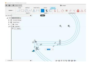
14. If all needed parts of a model are drawn, to create the 3D model it is necessary to exit from the sketch mode (*Finish Sketch* command). To apply *Extrude* or *Revolve* commands all the surfaces have to be closed (all lines connected).
