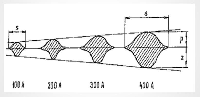
S - width of the bead p - height, z - depth penetration
