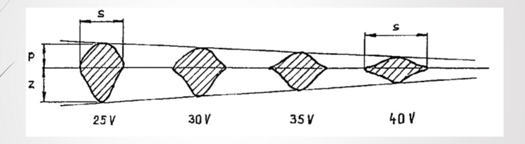
S - width of the bead p - cant of - penetration depth
