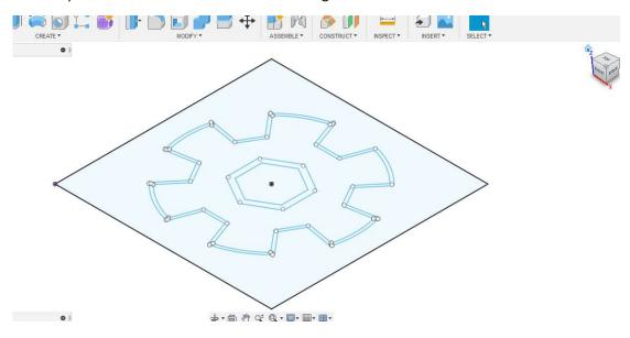
20. With the *Extrude* command we build the 3D model (pull the surface into space). It is necessary to choose closed surfaces. By entering the values or by pulling the blue arrow we define the thickness of the border.
