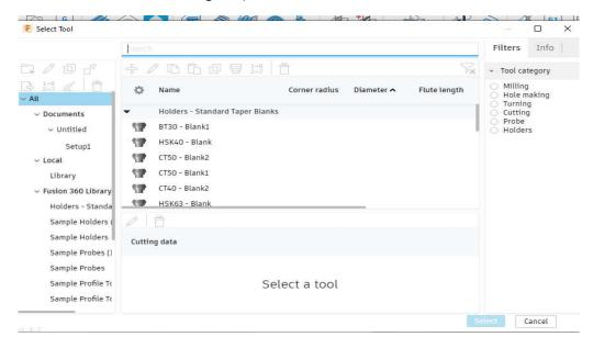
29. By clicking on the right mouse button over the option and selecting *Edit Tool* command we can change cutting tool and tool holder dimensions.
