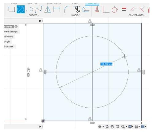
9. With the *Line* command it is possible to draw the contour of the model. We can draw all object lines at once. Using just a left mouse click, the command remains active, and we can draw the next desired line. With the *ESC* key we turn off the line command.
