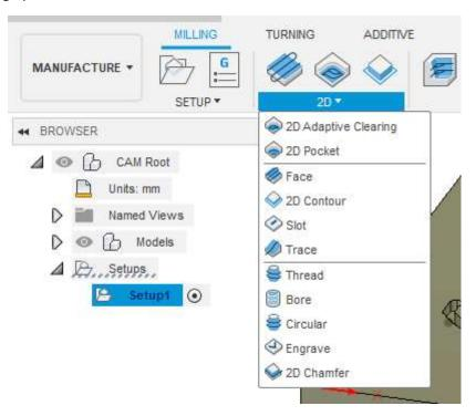
27. Choosing the **2D contour** milling option opens the window for setting up the cutting speed and ways of entering the cutting tool into the material. It is necessary to mark the contour on the 3D model. To finish the operation we need to choose the cutting tool.
