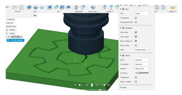
31. After reviewing the simulation, if no errors are shown, we can proceed to the generation of NC code through the *Post Process* option from the *Actions* menu. A window opens where we can choose the type of machine and the type of program on the computer.
