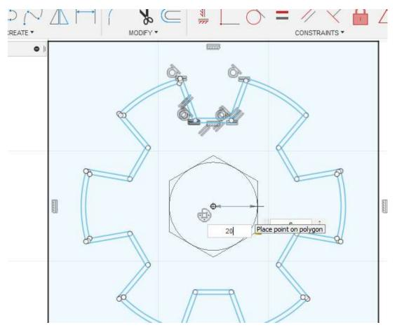
17. If all needed parts of a model are drawn, to create the 3D model it is necessary to exit from the sketch mode (*Finish Sketch* command). To apply *Extrude* or *Revolve* commands all the surfaces have to be closed (all lines connected).
