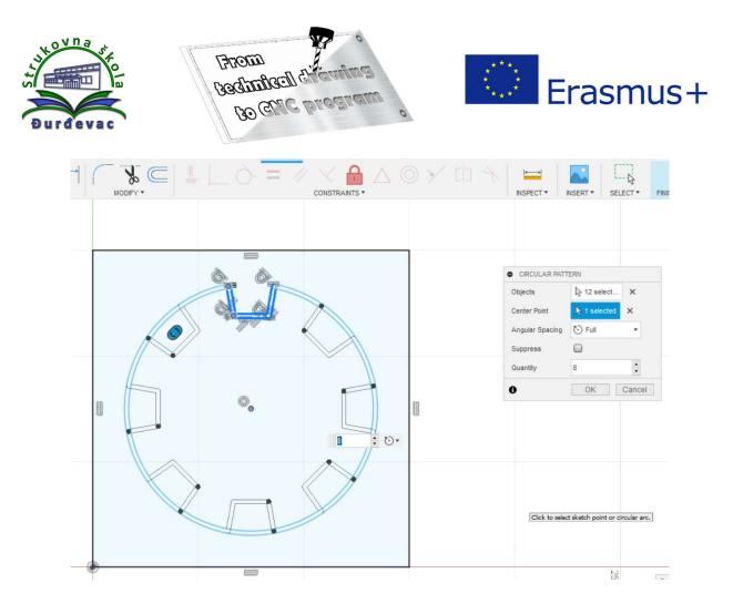
16. If all needed parts of a model are drawn, to create the 3D model it is necessary to exit from the sketch mode (*Finish Sketch* command). To apply *Extrude* or *Revolve* commands all the surfaces have to be closed (all lines connected).
