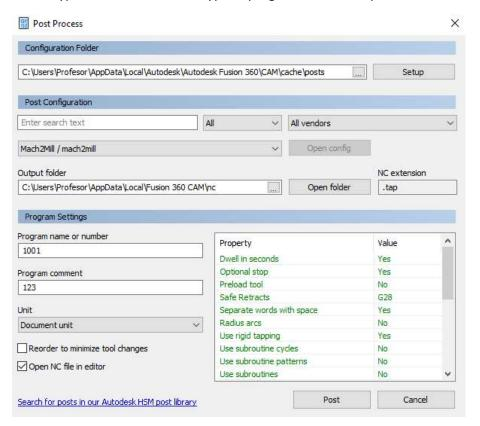
32. After all the settings, clicking on *Post* button opens a new window with the generated NC code, which we have to clean before we transfer it to the machine controller.
