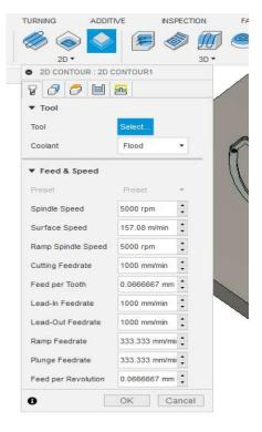
28. In the **Select Tool** window there is option to choose one of the tool from the list. By using filters it is possible to choose the tool and the tool holder. The tools can be adjusted if needed (e.g. different diameters of cutting tool).
