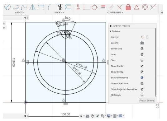
13. By using the *Trim* command it is possible to cut out part of lines or circles that we do not need anymore. If we want to delete an entire auxiliary line or circle, we need to select it first, then use the *Delete* key to delete it.
