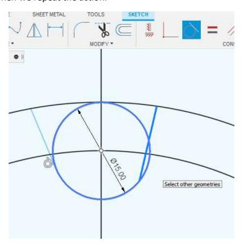
11. After placing all the lines tangently to the circle, we can use the *Dimension* command to determine the angles of inclination.
