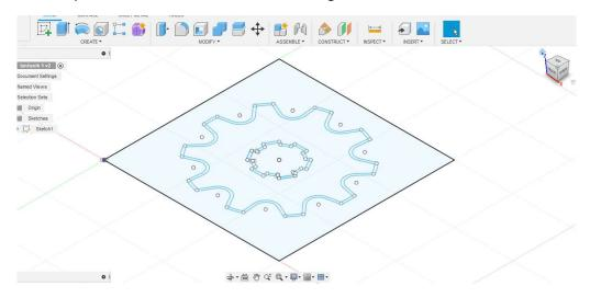
22. With the *Extrude* command we build the 3D model (pull the surface into space). It is necessary to choose closed surfaces. By entering the values or by pulling the blue arrow we define the thickness of the border.
