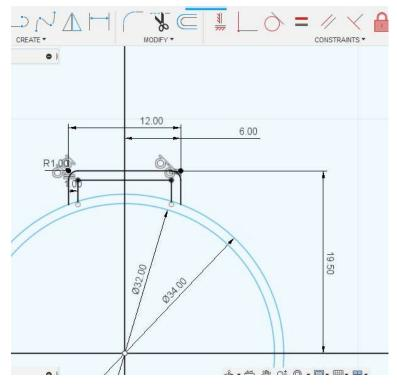
18. If we need to extend a line or circle to the next line or circle using it can bed one by using the *Extend* command. The part that will be extended will be shown in red.
