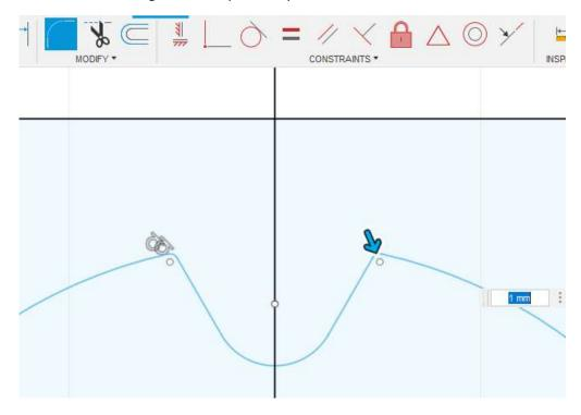
15. By using the *Offset* command it is possible to copy curves, which can speed up work during the drawing process.
