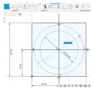
9. With the *Line* command it is possible to draw the contour of the model. We can draw all object lines at once. Using just a left mouse click, the command remains active, and we can draw the next desired line. With the *ESC* key we turn off the line command.
