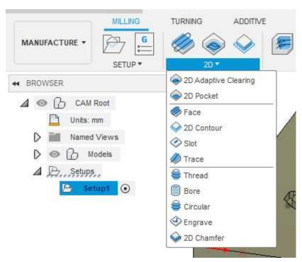
29. Choosing the **2D contour** milling option opens the window for setting up the cutting speed and ways of entering the cutting tool into the material. It is necessary to mark the contour on the 3D model. To finish the operation we need to choose the cutting tool.
