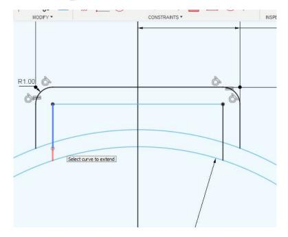
19. If all needed parts of a model are drawn, to create the 3D model it is necessary to exit from the sketch mode (*Finish Sketch* command). To apply *Extrude* or *Revolve* commands all the surfaces have to be closed (all lines connected).
