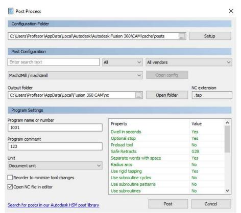
34. After all the settings, clicking on *Post* button opens a new window with the generated NC code, which we have to clean before we transfer it to the machine controller.
