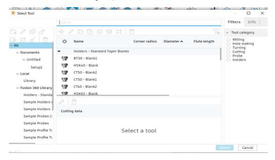
31. By clicking on the right mouse button over the option and selecting *Edit Tool* command we can change cutting tool and tool holder dimensions.
