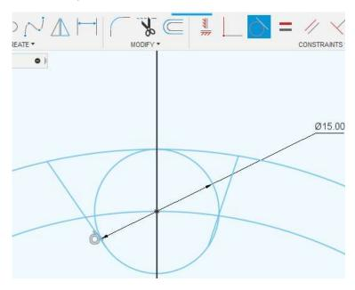
11. After placing all the lines tangently to the circle, we can use the *Dimension* command to determine the angles of inclination.
