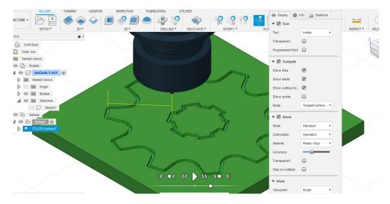
33. After reviewing the simulation, if no errors are shown, we can proceed to the generation of NC code through the *Post Process* option from the *Actions* menu. A window opens where we can choose the type of machine and the type of program on the computer.
