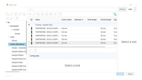
25. By clicking on the right mouse button over the option and selecting *Edit Tool* command we can change cutting tool and tool holder dimensions.
