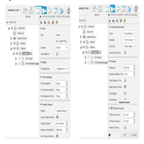
27. After setting all of the necessary options the simulation can be started by choosing the *Simulate* command from the *Actions* menu.
