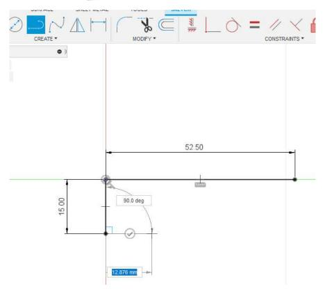
7. After drawing all the lines, we can use the *Dimension* command to determine the dimensions of the lines or circles. If the dimension is already visible, with a double click we have the option to change the dimension.
