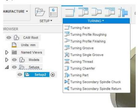
22. With *Face* option we can align the forehead of the material. A window opens where we can adjust the depth of cut, ways of approaching and moving the tool away from the workpiece.
