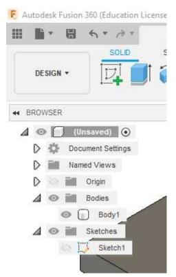
16. From the **Design** menu, by choosing the **Manufacture** option, it is possible to switch to the mode for making of the simulation and generating the NC code.
