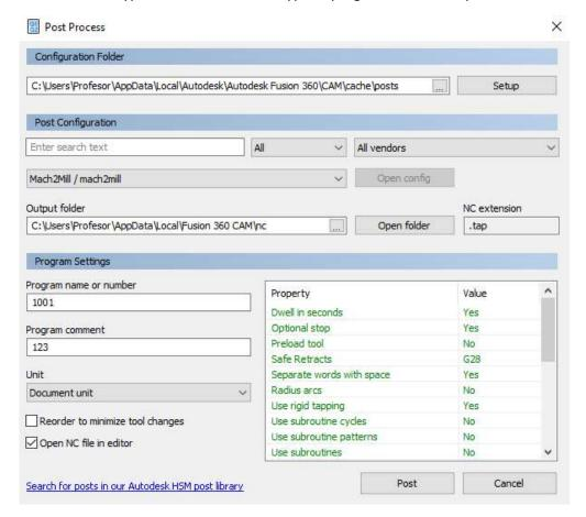
28. After all the settings, clicking on *Post* button opens a new window with the generated NC code, which we have to clean before we transfer it to the machine controller.
