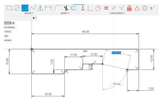
7. After drawing all the lines, we can use the *Dimension* command to determine the dimensions of the lines or circles. If the dimension is already visible, with a double click we have the option to change the dimension.
