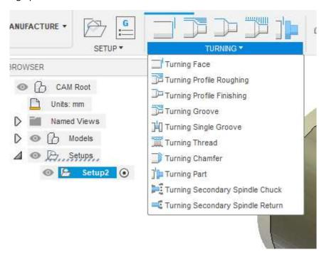
21. With *Face* option we can align the forehead of the material. A window opens where we can adjust the depth of cut, ways of approaching and moving the tool away from the workpiece.
