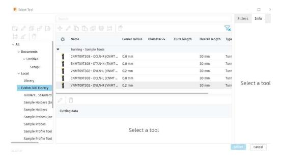
24. By clicking on the right mouse button over the option and selecting *Edit Tool* command we can change cutting tool and tool holder dimensions.
