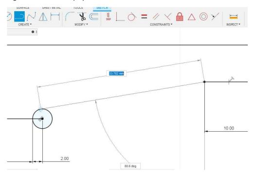
11. By using the *Trim* command it is possible to cut out part of lines or circles that are not needed anymore. If we want to delete an entire auxiliary line or circle, we need to select it first, then use the *Delete* key to delete the entire line or circle.
