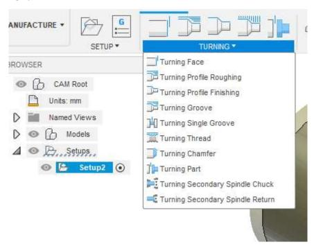
23. With *Face* option we can align the forehead of the material. A window opens where we can adjust the depth of cut, ways of approaching and moving the tool away from the workpiece.
