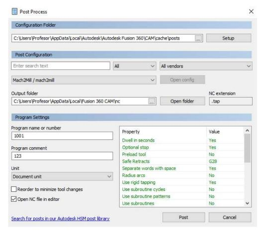
30. After all the settings, clicking on *Post* button opens a new window with the generated NC code, which we have to clean before we transfer it to the machine controller.
