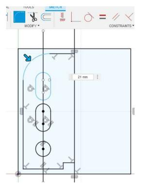
14. By using the *Offset* command it is possible to copy curves, which can speed up work during the drawing process.
