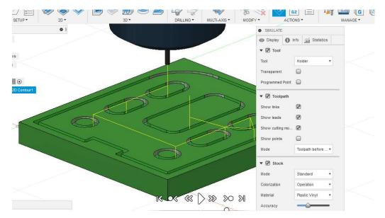
31. After reviewing the simulation, if no errors are shown, we can proceed to the generation of NC code through the *Post Process* option from the *Actions* menu. A window opens where we can choose the type of machine and the type of program on the computer.
