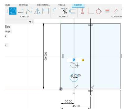
9. With the *Line* command it is possible to draw the contour of the model. We can draw all object lines at once. Using just a left mouse click, the command remains active, and we can draw the next desired line. With the *ESC* key we turn off the line command.
