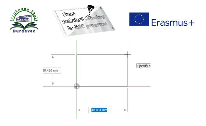
7. By using the *Sketch Dimension* command it is possible do define the length of line or a diameter of the circle and where we want to draw it, as well as make and show the exact dimensions from the coordinate system origin. If there are bisectors in the drawing, we can draw them as auxiliary lines for easier positioning of other lines or circles and delete them later.
