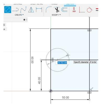
9. With the *Line* command it is possible to draw the contour of the model. We can draw all object lines at once. Using just a left mouse click, the command remains active, and we can draw the next desired line. With the *ESC* key we turn off the line command.
